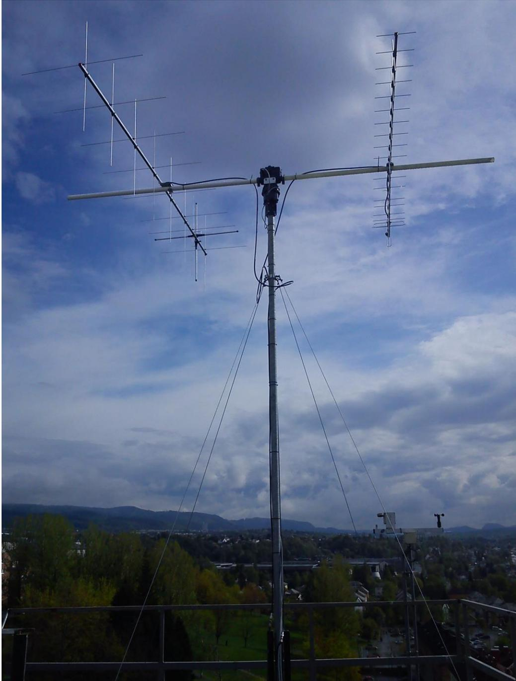
Fuente: Antenna system for a ground station communicating with the NTNU Test Satellite (NUTS), July 2011.
