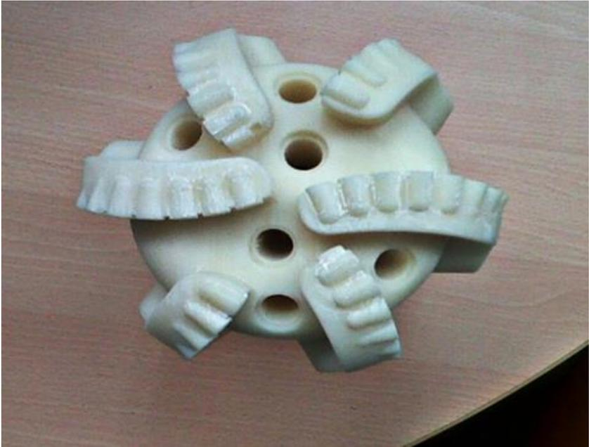
**Figuras 42. DISEÑO EN IMPRESORA 3D UNA BROCA TIPO PDC**
