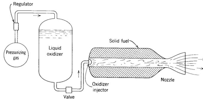
Figure 3.5: Hybrid rocket engine configuration. From [59]
