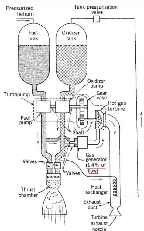
Figure 3.3: Liquid propulsion configuration. From [59]
