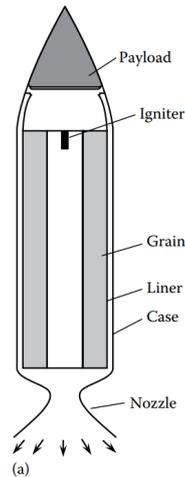
Figure 3.4: Solid rocket engine configuration. From [36]
